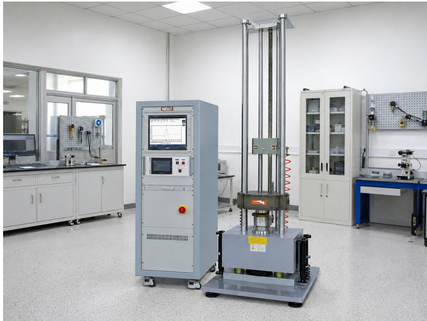
Typical laboratory installation of the HSKT10 mechanical shock test system
