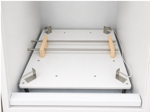
Close-up of the internal Annex D-oriented fixture
