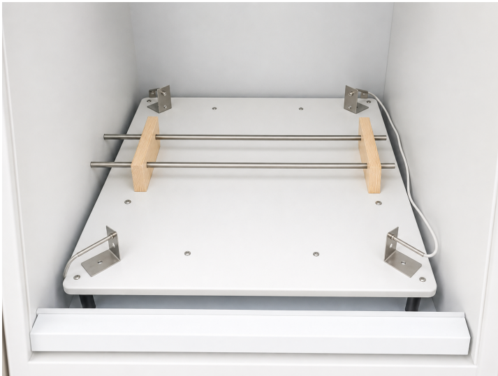
Internal platform, specimen supports and temperature-measurement brackets
