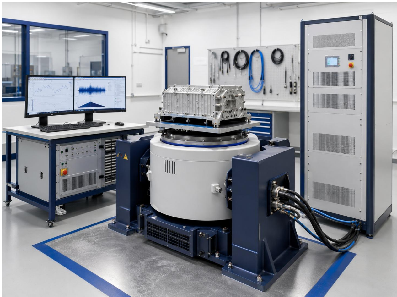
Figure 1. Complete vibration test system laboratory setup, including shaker, controller workstation, amplifier cabinet, cables and mounted test fixture.
