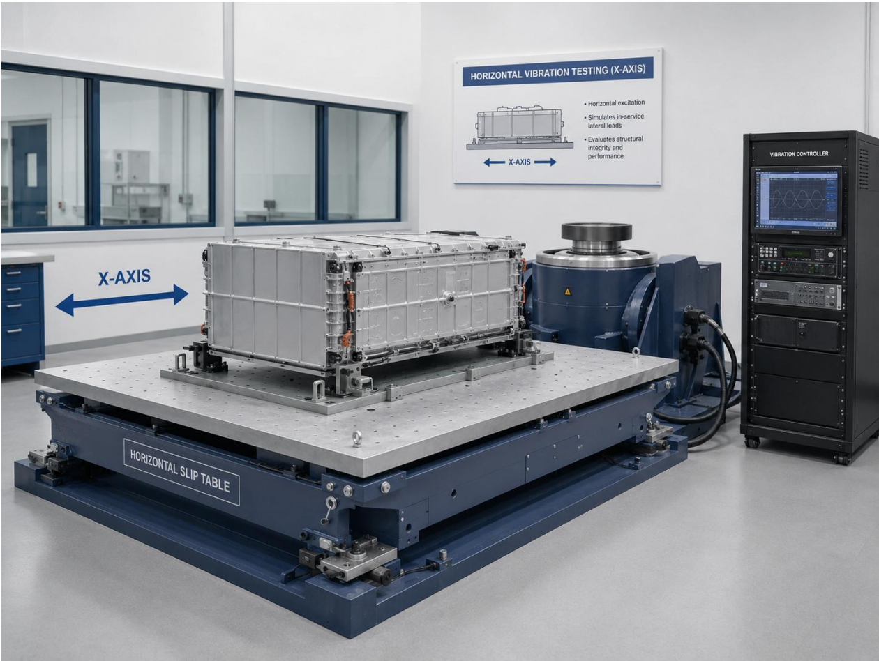
Figure 4. Horizontal slip table vibration test system for X-axis testing with a battery module, shaker and vibration controller.
