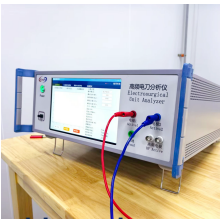
KP8850 front panel with touchscreen and electrode ports
